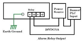
The failure events are selectable and enabled using the DIP switch on the ES8105. The relay contacts are rated for a maximum of 1A at 24VDC.
