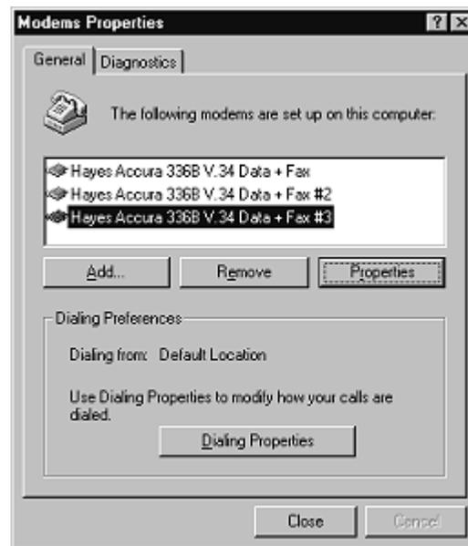
12. If you need to configure modem properties (maximum baud rate, data bits, parity, and so on), click the **Properties** button, make the needed changes, then click **OK** to return to this window.
