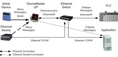
EtherNet/IP Filtering Functionality (V3.x)
