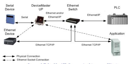
Comtrol EtherNet/IP System Architecture (V3.x)
