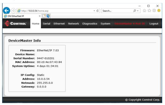
The *Home* page displays the DeviceMaster information including the firmware version, device name, serial number, MAC address and current network configuration..
