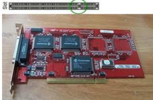
This slot will accept either the RocketPort PCI, RocketPort uPCI or the RocketPort Infinity
