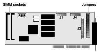
If you have a 16-port card, the jumper blocks for Ports 9 through 16 are located on the upgrade module.
