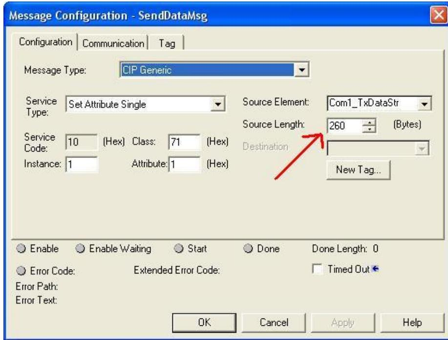
The **Source Length** of the MSG instruction must be long enough to transfer the full transmit data message. This includes the 4 byte sequence number/length header and the length of data.
