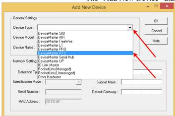
You will now need to define the device. In this example we are installing a 1 port DeviceMaster RTS 5VDC model. Click the drop down arrow on Device Type: and select the DeviceMaster RTS.
