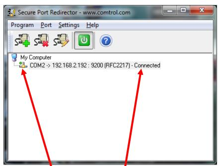
Once the serial port is opened, the line will look like what is seen in this graphic. This shows an active connection from the Test Terminal application. Note the "Green Dot" and "Connected"
