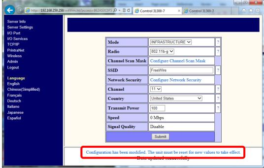
Click on the notice: Configuration has been modified. The unit must be reset for new values to take effect.
