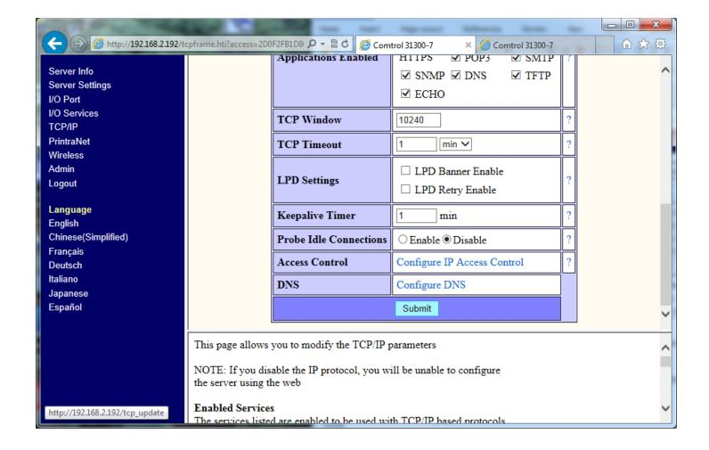
New line "Configuration has been modified. The unit must be reset for new values to take effect." Click this to reboot FreeWire.
