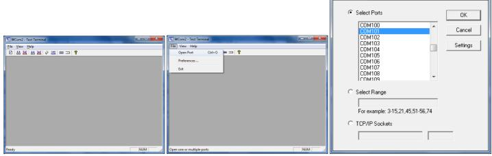
In Test Terminal Select the "File" drop down menu and select "Open Port" and select the first com number added in SPR (Secure Port Redirector).
