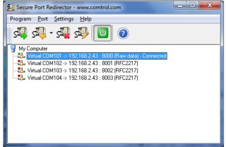
If you return to SPR (Secure Port Redirector) you should see that the port is open. This is showing that we are in the process of testing the first com port using Test Terminal. The Red Dot will now be Green and it will show 'Connected' on ports that are currently in use.
