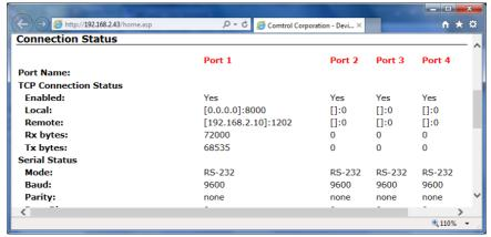
Open the web page and you will see the IP address of the PC that Test Terminal is running in and the Rx and Tx bytes should be incrementing. You may need to refresh the web page a few times to see changes take place.
