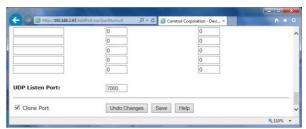
Scroll to the bottom of the page. If the serial settings for all ports are the same you make select the "Clone Port" option. Otherwise leave it blank and open each port individually to set the serial settings and Enable options.
