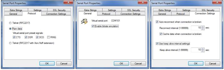
Set all tabs as shown here for initial connections and testing. See the help system if you need to modify these.
