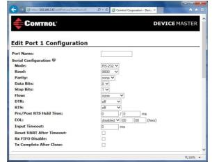
Open a web browser to the DeviceMaster and click on Port 1 to open the set "Edit Port 1 Configuration page. Set the serial port settings to agree with the device attached to the DeviceMaster physical serial port 1. If the defaults are acceptable you can skip to the next step. If the settings need changing open each serial port individually to make changes as necessary.
