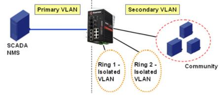
This figure shows a typical private VLAN network. A SCADA/Public Server or NMS workstation is usually located in a primary VLAN. Client PCs and rings are usually located within the secondary VLAN.
