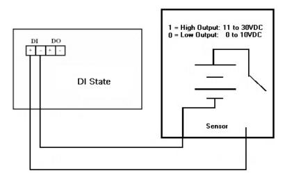
Digital output relay contacts are energized (open) for normal operation and close for fault conditions. The digital output relay contacts support up to 1A at 30VDC. Do not apply voltage and current higher than the specifications.
