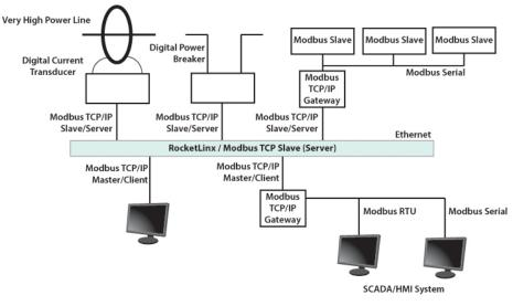
The ES8509-XT operates as slave/server device, while a typical master/client device is a host computer running appropriate application software, for example, a SCADA / HMI system. The ES8509-XT can be polled through Ethernet, thus the Modbus TCP/IP master can read or write to the Modbus registers provided by the Modbus TCP/IP.
