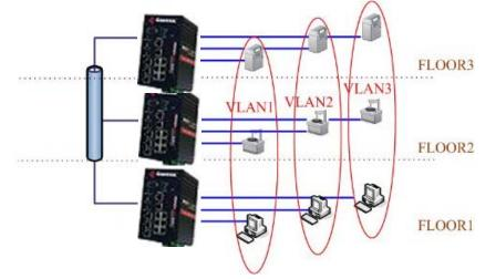
The ES8509-XT supports VLAN tunneling (QinQ), which expands the number of VLANs by adding a tag to the 802.1Q packets. The original VLAN is usually identified as Customer VLAN (C-VLAN) and the new VLAN is Service VLAN(S-VLAN). By adding the additional tag, QinQ increases the possible number of VLANs. After QinQ is enabled, the ES8509-XT can reach up to 256x256 VLANs. With different standard tags, it also improves network security.
