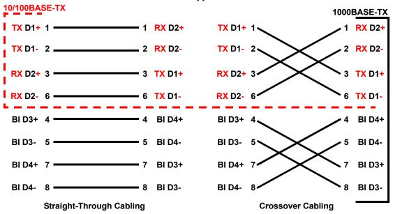
Connect one side of an Ethernet cable into any switch port and connect the other side to your attached device. The **LNK/ACT** LED is lit when the cable is correctly connected. Always make sure that the cables between the switches and attached devices (for example, switch, hub, or workstation) are less than 100 meters (328 feet) and meet these requirements.
