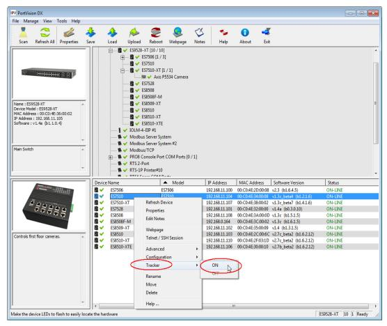
2. If necessary, you may need to click Tracker and ON several times to catch the flashing SYS LED.
