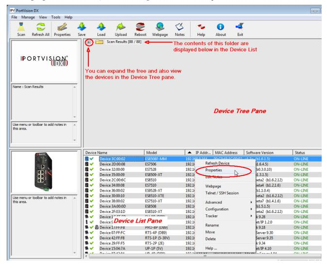
5. Optionally, rename the ES7510-XT in the **Device Name** field for a PortVision DX friendly name. The default name displays as *Device* and the last three sets of hex numbers from the MAC address.
