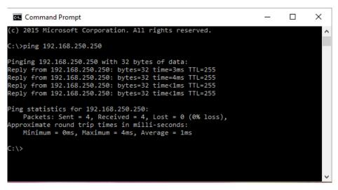
Note: If you did not program the IP address for your network using PortVision DX (Configuring the Network Settings on Page 20), you need to change your computer IP address to 192.168.250.x (Network Mask: 255.255.0.0).
