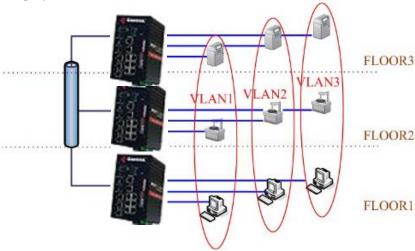
The ES7510-XT supports VLAN tunneling (QinQ), which expands the number of VLANs by adding a tag to the 802.1Q packets. The original VLAN is usually identified as Customer VLAN (C-VLAN) and the new VLAN is Service VLAN(S-VLAN). By adding the additional tag, QinQ increases the possible number of VLANs. After QinQ is enabled, the ES7510-XT can reach up to 256x256 VLANs. With different standard tags, it also improves network security.
