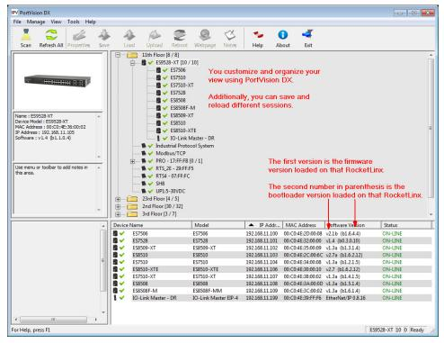
4. Check the <u>Comtrol download</u> site for the latest firmware and bootloader. Simply, click your product type and click the <u>Software</u> link and check the latest version against the version on the ES7510-XT.
