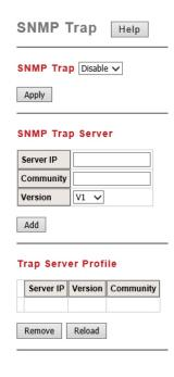
You can see the change of the SNMP predefined standard traps and Comtrol pre-defined traps. The predefined traps can be found on the Comtrol ftp site.
