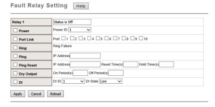
The **Relay 1** field shows the current state of the relay. If the relay is triggered, the event type is marked with an asterisk (\*). The above image shows that a power event occurred.
